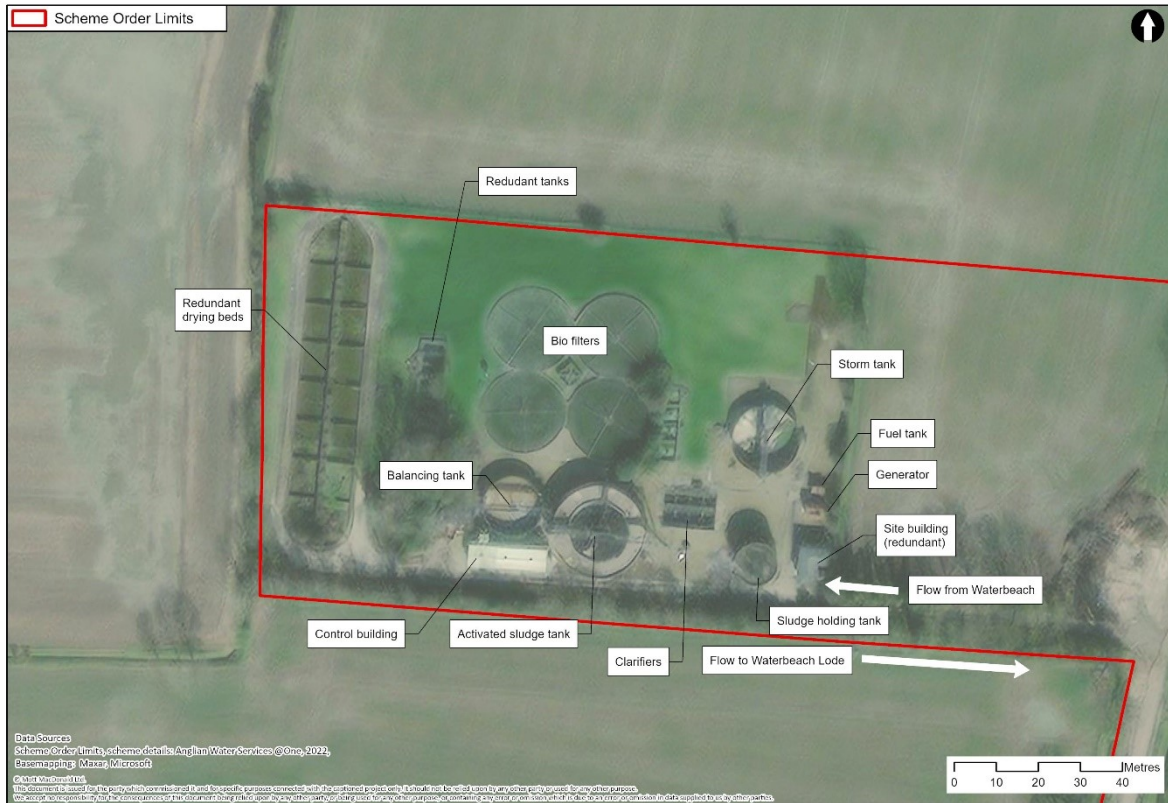
Figure 8.3: Schematic of the Waterbeach WRC
